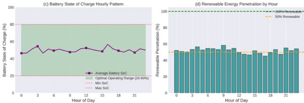
Figure 3. Diurnal performance patterns: (a) average daily generation profiles for solar PV and wind power with standard deviation bands; (b) total renewable generation versus grid load demand with surplus/deficit regions; (c) mean battery state of charge by hour with optimal operating range; (d) renewable energy penetration rate by hour of day.
