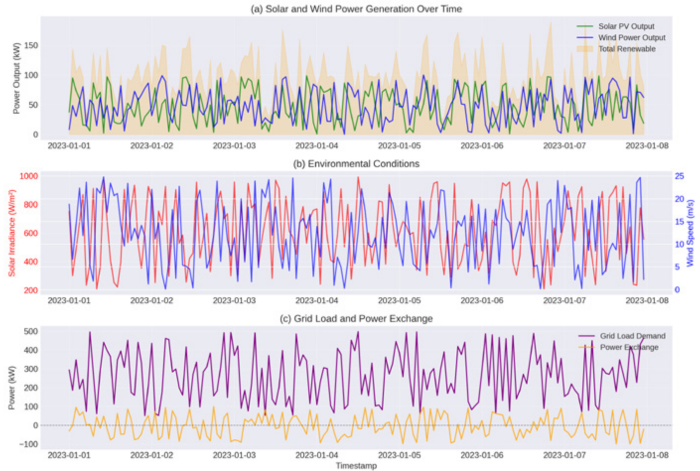
Figure 1. Hybrid system performance time series analysis: (a) solar PV and wind power output with total renewable generation overlay; (b) concurrent solar irradiance and wind speed profiles; (c) grid load demand and bidirectional power exchange.
